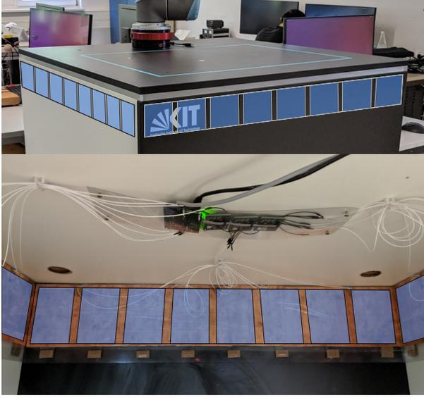
Fig. 2: Capacitive proximity sensors installed in the table
