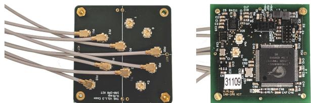
Fig. 1: CTPS module. Top and bottom side
